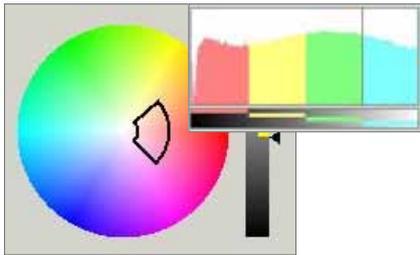
Color images are represented by the HSI color model and the hue, saturation and intensity ranges of pixels can be used to define a phase.
