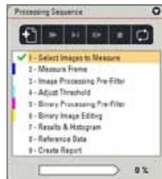
Once the parameters are established, they are saved to a named configuration file. This can then be applied to multiple sets of specimen images to ensure that repeatable and reproducible analysis is performed.
