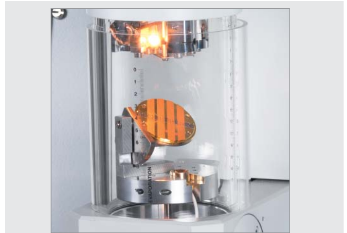
Carbon rod evaporation of specimens on grids using a tiltable stage.
